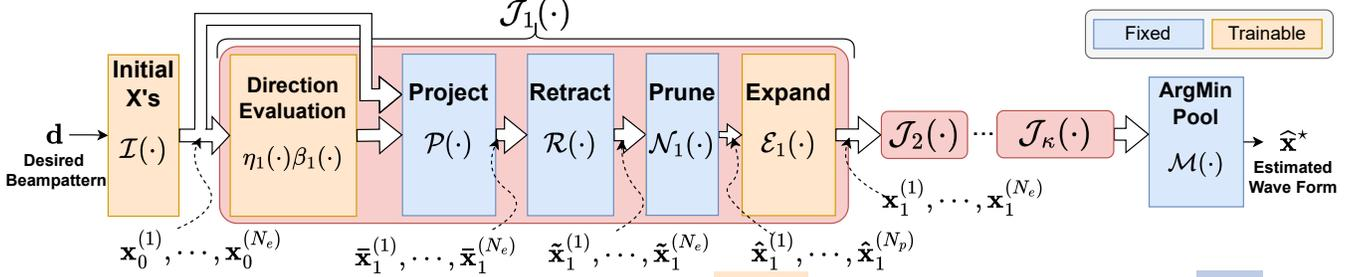
**Fig. 2.** Proposed FLI Architecture. Trainable blocks are colored in Orange and blocks with fixed parameters in Blue.
