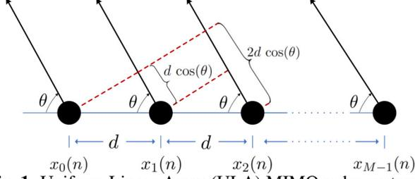
**Fig. 1.** Uniform Linear Array (ULA) MIMO radar system
